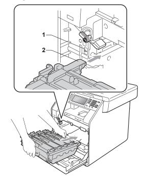
Turn the green lock lever (1) clockwise to the lock position.
